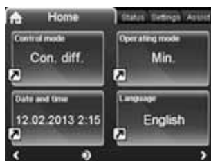
Fig. 16 Example of main display on a TPE Series 2000 with advanced control panel
